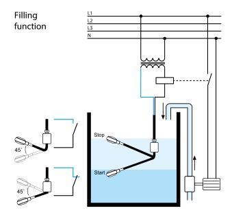
When black and blue/grey wires are used, the circuit opens when the float is up and closes when the float in down. In this case the brown wire must be insulated.
