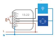
Special function RIa - Step relay (switch control). Ideal for converting a traditional system using one, two, or four way switches, into a Smart system
